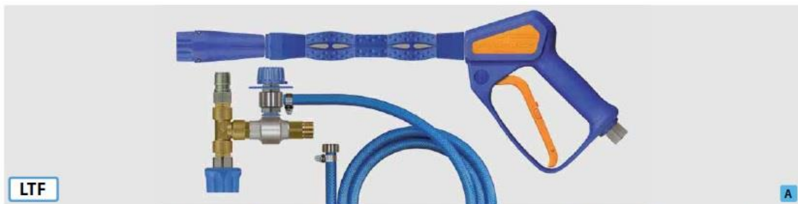
easywash365+ foam set: easywash365+ foam lance standard with foam head ST-75, injector ST-160 (Coupling ST-45-250 nickel-plated brass, plug ST-45-250 zinc-plated steel and M22 M) with metering valve ST-161, suction hose 1000 mm and suction filter ST-32. Max. 250 bar / 90 °C
