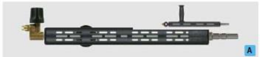
Plug KW. Lance with insulation ST-9 & grip, valve ST-53 on top and low pressure nozzle. Max. 250 bar / 150 °C
