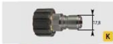
Plug : F. Stainless steel + brass. Max. 250 bar / 150 °C
