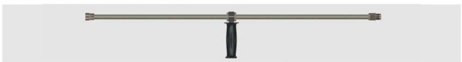
1/2" M. Lance with grip and sleeve 1/4" F NPT stainless steel without high pressure nozzle. Max. 600 bar / 150 °C
